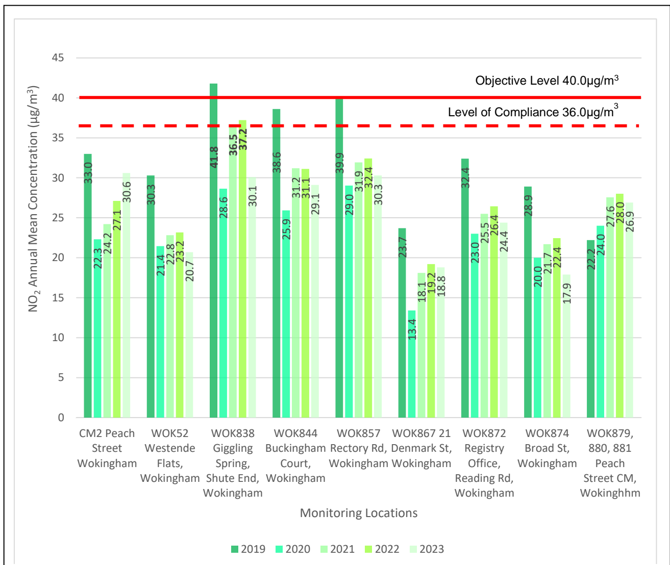
Figure 3.4 Trends in Annual Mean NO 2 Concentrations within the Wokingham Town Centre AQMA from 2019 to 2023.
